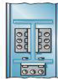
typical "fixed-supported" connection (metal) (b)
